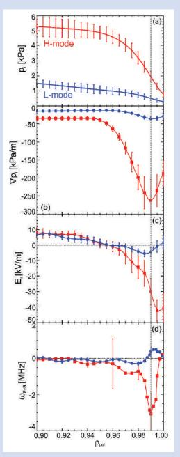
Fig. 1: (a) Main ion pressure and its gradient (b), (c) radial electric field and (d)  $\mathbf{E} \times \mathbf{B}$  velocity shear.
