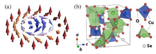
Fig. 1: (a) Schematic illustration of magnetic skyrmion. (2) Crystal structure of chiral-lattice multiferroic insulator Cu<sub>2</sub>OSeO<sub>3</sub>,
