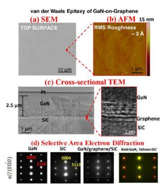
Figure 2. 3D-on-2D technology as exemplified by GaN-on-Graphene. High quality GaN layers are grown on epitaxial graphene. (a) Scanning electron and (b) atomic force microscopy images reveal atomically smooth surfaces. (c) Cross-sectional transmission electron microscopy and (d) selective area electron diffraction reveal crystallographic arrangement between the layers. [adopted from Nat. Comm. 5: 4836 (2014)]
