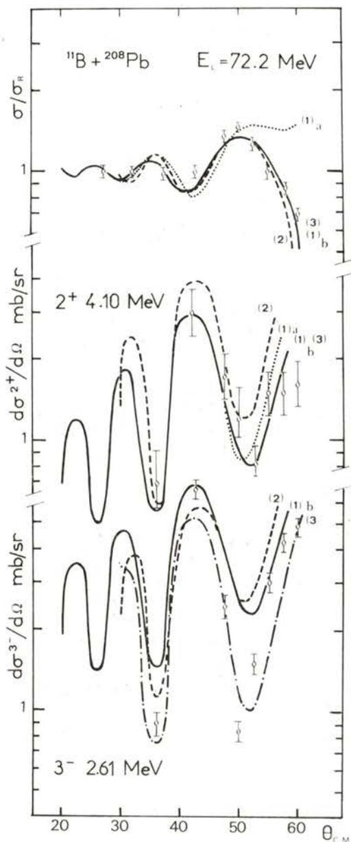
Fig. 3 — Cross-sections of the elastic and inelastic  $2^+$  (4.10 MeV) and  $3^-$  (2.61 MeV) excitation of  $^{208}\text{Pb}$  in scattering of  $^{11}\text{B}$  on  $^{208}\text{Pb}$  at  $E_L = 72.2$  MeV. Potentials (1) and (2) give similar fits to the data; potential (3) gives a better agreement with the experimental results [9] for the  $3^-$  excitation. The uniform approximation (b) for the elastic and inelastic  $2^+$  cross-sections are compared to the asymptotic expressions (a)
