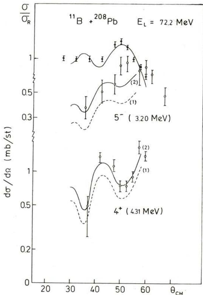
Fig. 4 — Cross-sections of elastic and inelastic  $5^- (3.20 \text{ MeV})$  and  $3^+ (4.31 \text{ MeV})$  excitation of  $^{208}\text{Pb}$  in scattering of  $^{11}\text{B}$  on  $^{208}\text{Pb}$  at  $E_L = 72.2 \text{ MeV}$ . Potentials (1) and (2) are the same of Figure 3.
