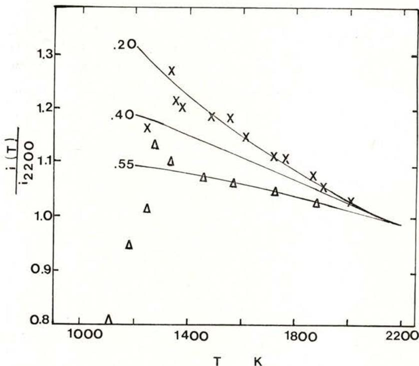
Fig. 4—Data for Sodium ionization on cleaned Iridium surface (X) and on Iridium with adsorbed oxygen ( $\Delta$ ). Lines represent the theoretical behaviour of  $i(T)/i(2200$  K) for several values of  $\phi_i - I$
