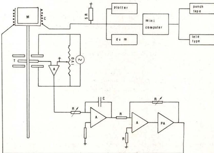
Fig. 3 — Sketch of the magnetometer and the corresponding logging system.
