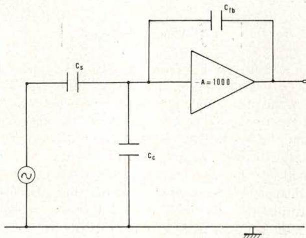
Fig. 2 — Input amplifier used as a 'virtual ground amplifier'.
