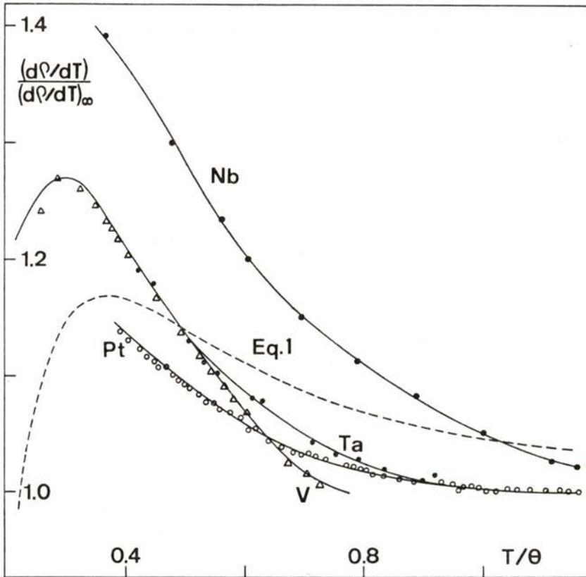
Fig. 3 — Normalised thermal derivative  $(d\rho/dT)/(d\rho/dT)_\infty$  as a function of  $(T/\theta)$  for Nb, V, Ta, Pt. The dashed curve was obtained from differentiation of expression (1).
