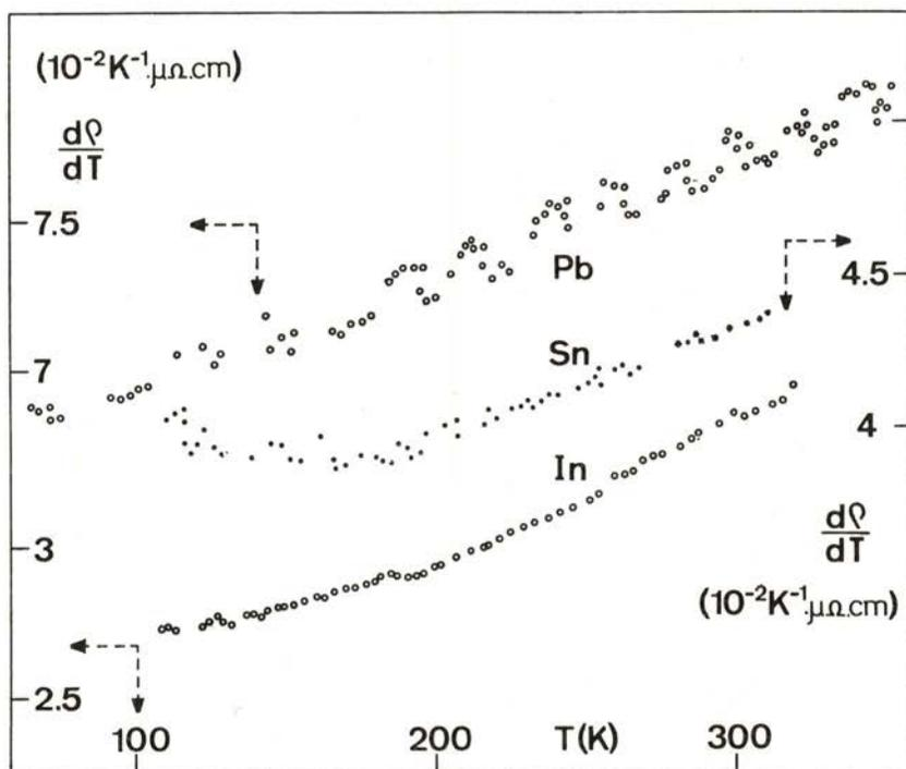
Fig. 4 — Thermal derivative,  $d\rho/dT$ , as a function of the temperature for the low melting point metals In, Sn and Pb.
