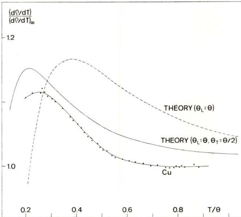
Fig. 2 — Normalised thermal derivative  $(d\rho/dT)/(d\rho/dT)_\infty$  as a function of  $(T/\theta)$ ; the dashed curve was obtained from differentiation of expression (1), while the full curve was derived from expression (2), in which two maxima in the density of states of the phonon spectrum are considered. The third curve presents the experimental results obtained for Cu.
