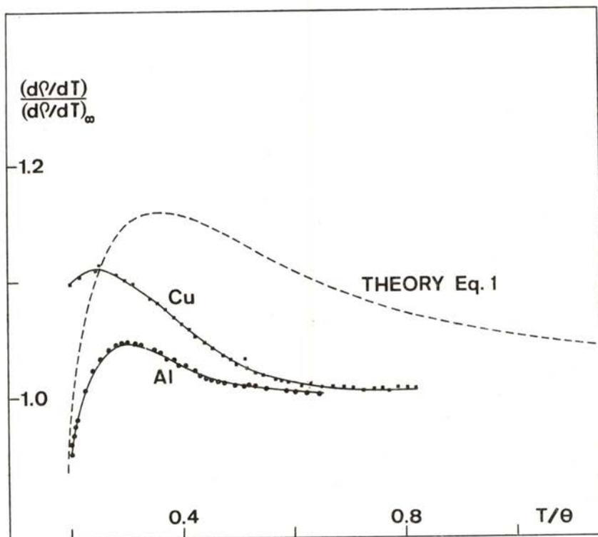
Fig. 1 — Normalised thermal derivative  $(d\rho/dT)/(d\rho/dT)_\infty$  as a function of normalised temperature  $(T/\Theta)$  for Cu and Al. The dashed curve represents  $(d\rho/dT)/(d\rho/dT)_\infty$  obtained from differentiation of expression (1).
