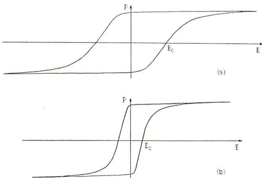
Fig. 7 — Hysteresis loops relating to sample 1 (a) at temperature  $T = 319.75\text{K}$  and sample 3 (b) at temperature  $T = 319.85\text{K}$ . The coercive fields are  $E_c$  (a)  $= 3,9 \text{ kV/cm}$  and  $E_c$  (b)  $= 0,7 \text{ kV/cm}$ , respectively.
