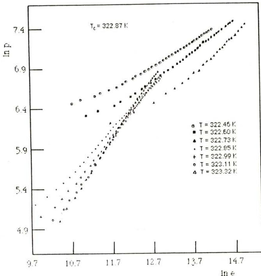
Fig. 8 —  $\ln p$  vs.  $\ln e$  relating to sample 3, for the indicated temperatures, with  $T_c = 322.87\text{K}$ .
