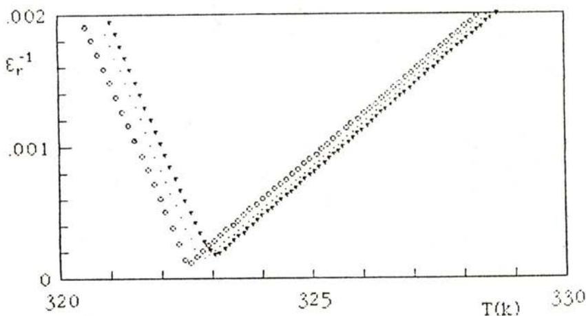
Fig. 3 — Inverse of relative dielectric constant  $\epsilon_r^{-1}$  vs. temperature  $T$ , for three consecutive heatings relating to sample 3:  $\circ \rightarrow$  heating on virgin sample;  $\bullet \rightarrow$  first heating on monodomain sample;  $\blacktriangledown \rightarrow$  third heating on monodomain sample.
