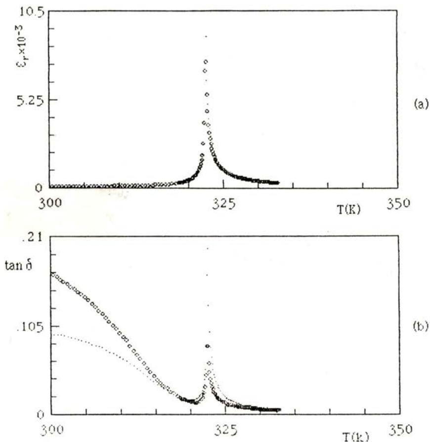
Fig. 4 — Relative dielectric constant  $\epsilon_r$  vs. temperature  $T$  (a) and loss tangent  $\tan \delta$ , vs.  $T$  (b) relating to virgin sample 3. These measurements were taken when heating the sample at the frequency of:  $\bullet \rightarrow 1$  kHz;  $\circ \rightarrow 10$  kHz.
