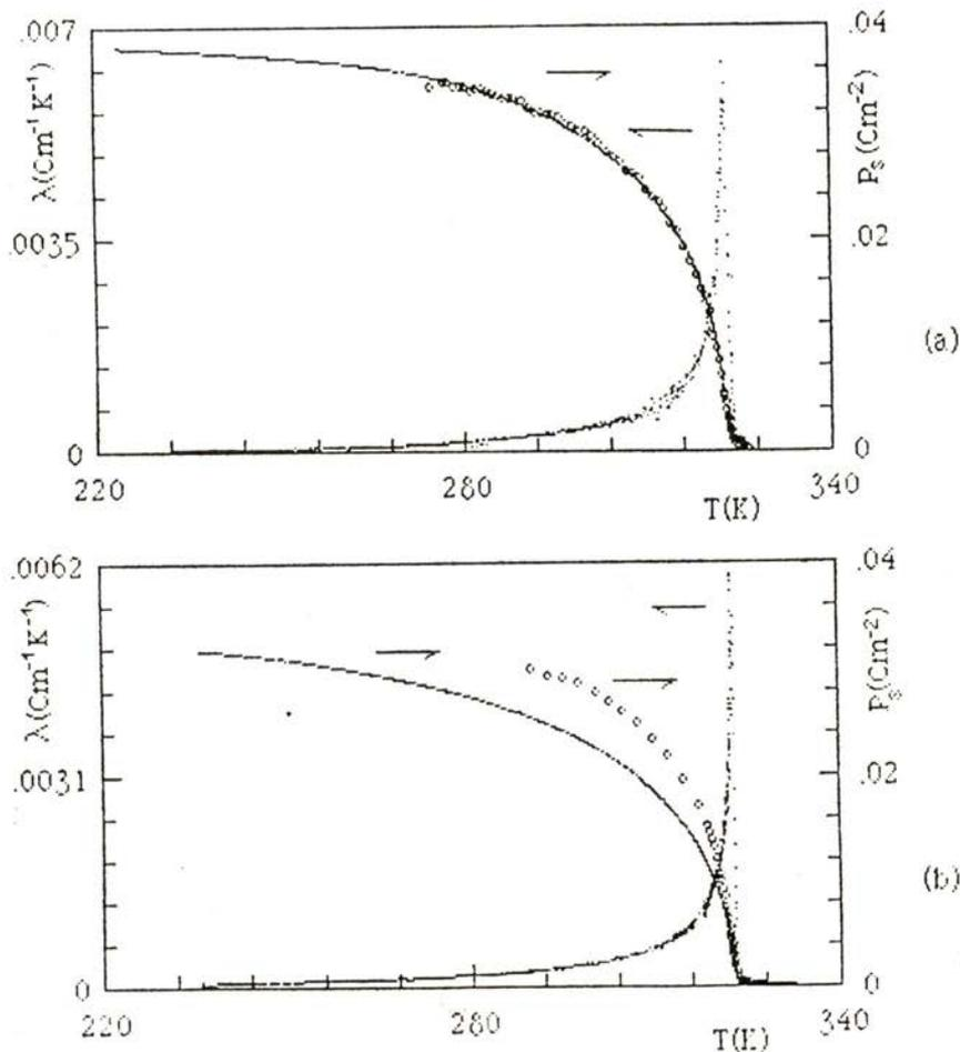
Fig. 6 — Spontaneous polarization  $P_s$  and pyroelectric coefficient  $\lambda$  vs. temperature  $T$  on sample 1 (a) and on sample 3 (b).  $\bullet \rightarrow \lambda$  vs.  $T$ ;  $\circ \rightarrow P_s$  vs.  $T$ , obtained from hysteresis loops;  $- \rightarrow P_s$  vs.  $T$ , obtained from integration of  $\lambda$ .
