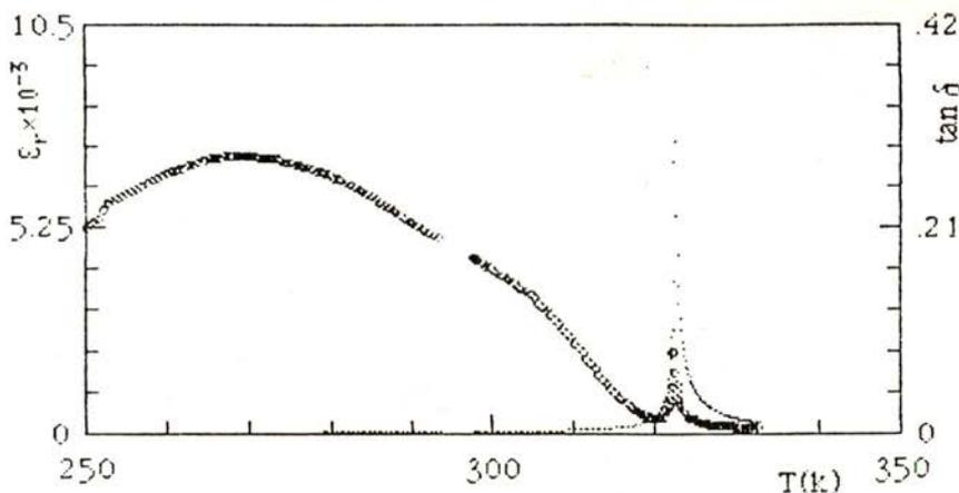
Fig. 5 — Measurements of  $\epsilon_r$  vs. T (•) and  $\tan \delta$  vs. T (o) relating to sample 3. The virgin sample was cooled from room temperature to  $\sim 250$ K and then heated at the frequency of  $\sim 10$  kHz. The data acquisition was momentarily interrupted at around  $\sim 295$ K.
