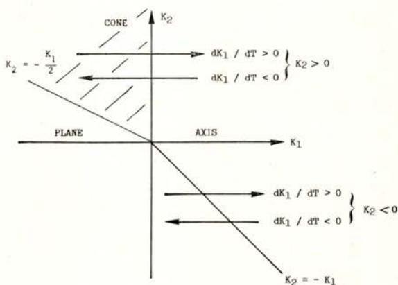
Fig. 1 — Spin reorientations in the  $K_2$ ,  $K_1$  plane
