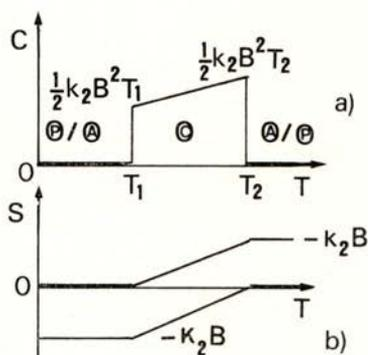
Fig. 2 — (a) Heat capacity for constant  $K_2 > 0$ , corresponding to  $B > 0$  (plane stable for  $T < T_1$ ) and  $B < 0$  (axis for  $T < T_1$ )
