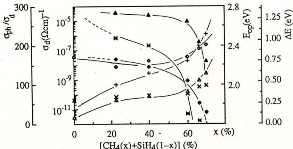
Fig. 6 - The dependence of  $\sigma_{ph}/\sigma_d$  (\*),  $\sigma_d$  (♦, ▲),  $E_{op}$  (+, △) and  $\Delta E$  (◇, ×) on the dilution ratio used for undoped (a-Si:C:H (\*, ♦, +, ◇)) and doped (a-Si:C(B):H (▲, △, ×)) samples produced at low powers, respectively.
