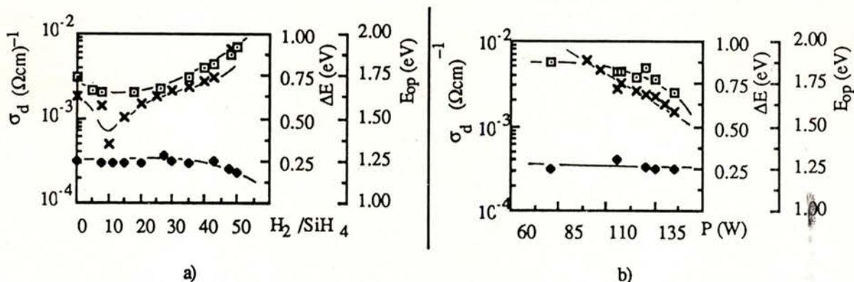
Fig. 7 - a) Dependence of  $\sigma_d$  ( $\times$ ),  $E_{op}$  ( $\square$ ) and  $\Delta E$  ( $\blacklozenge$ ) on  $\text{H}_2/\text{SiH}_4$ . b) The same dependence as a function of the power used.
