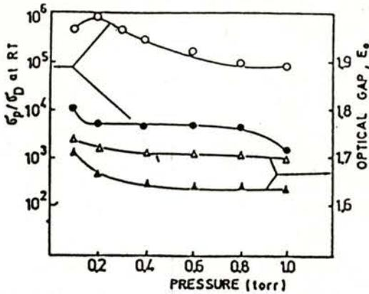
Fig. 4 - Dependence of  $\sigma_{ph}/\sigma_d$  and  $E_{op}$  on  $p$  for undoped films deposited by TCDDC system (o) and by a conventional diode-system (o).
