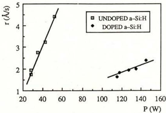
Fig.2 - Growth rate: as a function of power used for undoped (□) and doped (◆) (with Si<sub>4</sub>H<sub>2</sub> < 5 %) for a-Si:H films.
